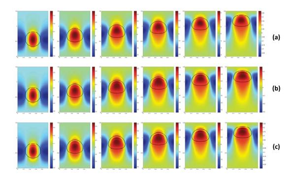
Figure 2: The vertical velocity component in the case of a lighter drop immersed in a heavier fluid with density ratio  $\rho_1$ :  $\rho_2 = 1$ : 50 at t = 0.6, 1.2, 1.8, 2.4, 3, 3.6. (a) M1, (b). M2, (c). M3. Each figure is superimposed by the shape of the drop, i.e. the zero contour curve of the phase-field function  $\phi$ , at the corresponding time.
