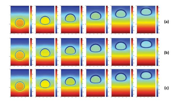
Figure 3: The pressure field in the case of a lighter drop immersed in a heavier fluid with density ratio  $\rho_1: \rho_2 = 1:50$  at t = 0.6, 1.2, 1.8, 2.4, 3, 3.6. (a) M1, (b). M2, (c). M3. Each figure is superimposed by the shape of the drop, i.e. the zero contour curve of the phase-field function  $\phi$ , at the corresponding time.
