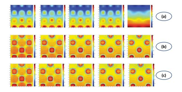
Figure 13: The hydrodynamic pressure p at t = 0.1, 0.2, 0.3, 0.4, 15 in the case of binary fluid mixing for all three models. (a) M1, (b) M2, (c) M3. The solutions nearly reach quasi-steady state at t = 15.
