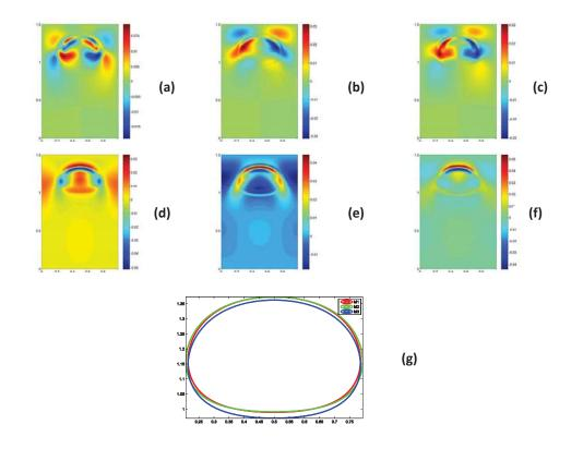
Figure 4: The velocity difference between pairs of the phase field models investigated. (a) u(M1) - u(M2), (b) u(M1) - u(M3), (c) u(M2) - u(M3), (d) v(M1) - v(M2), (e) v(M1) - v(M3), (f) v(M2) - v(M3), (g) Comparisons of the zero contour curves of  $\phi$  for all three models. The results are based on the solutions at t = 3.6.
