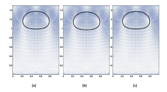
Figure 5: The velocity field superimposed by the shape of the drop at t = 3.6 for the three models. (a) *M*1 (b) *M*2, (c) *M*3.
