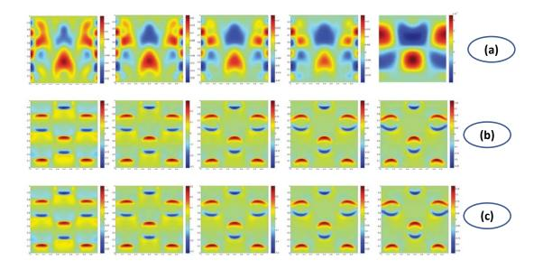
Figure 12: The velocity component v at t = 0.1, 0.2, 0.3, 0.4, 15 in the case of binary fluid mixing for all three models. (a) M1, (b) M2, (c) M3. The solutions nearly reach quasi-steady state at t = 15.
