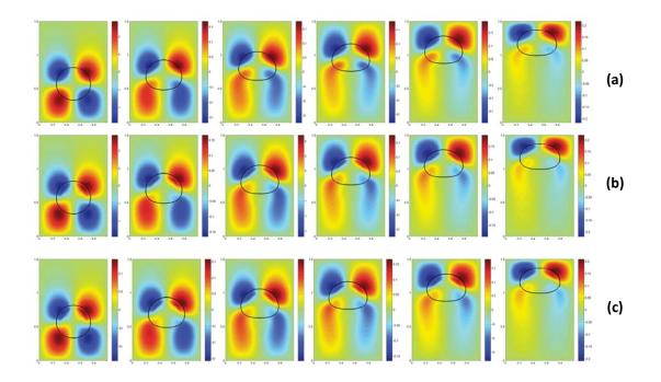
Figure 1: The horizontal velocity component in the case of a lighter drop immersed in a heavier fluid with density ratio  $\rho_1 : \rho_2 = 1 : 50$  at time t = 0.6, 1.2, 1.8, 2.4, 3, 3.6. (a) M1 (Model 1); (b). M2 (Model 2); (c). M3 (Model 3). Each figure is superimposed by the shape of the drop, i.e. the zero contour curve of the phase-field function  $\phi$ , at the corresponding time.
