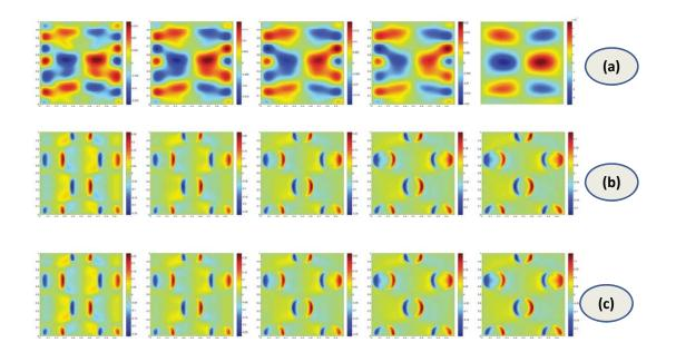
Figure 11: The velocity component u at t = 0.1, 0.2, 0.3, 0.4, 15 in the case of binary fluid mixing for all three models. (a) M1, (b) M2, (c) M3. The solutions nearly reach quasi-steady state at t = 15.
