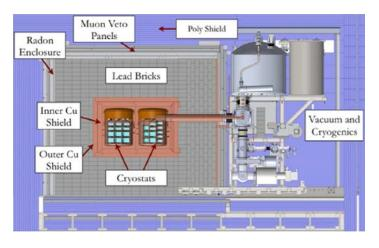
Schematic of the Majorana Demonstrator located at the Sanford Underground Research Facility (SURF) in Lead, South Dakota. The Demonstrator holds the Germanium crystals for our search for neutrinoless double beta decay.
