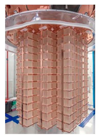
Tellurium crystals that make up the heart of the CUORE experiment at the Laboratori Nazionali del Gran Sasso in Assergi, Italy.
