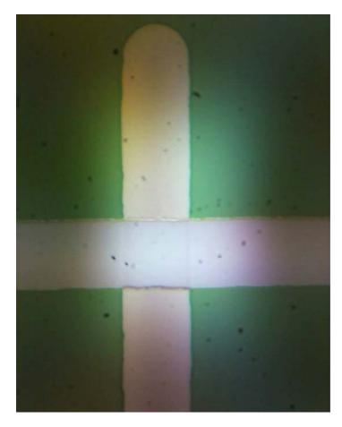
Optical microscopy image of a cross-bar array memristor.
