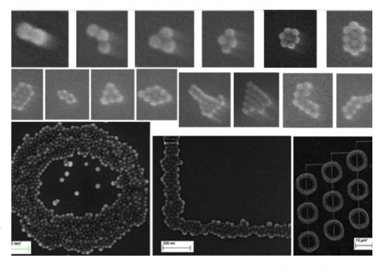
**Figure 1:** Example Scanning Electron Microscopy (SEM) images of magnetic nanoparticle self-assembly. **Top:** Random self-assembled patterns of 25 nm diameter magnetic nanoparticles. **Bottom:** Programmed assembly of nanoparticles into torii, rectangles, and more complex structures using recorded patterns on disk drive media.
