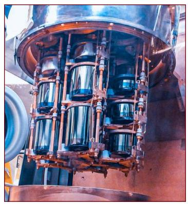
An inside look at the Germanium detectors used in the MAJORANA Demonstrator. The larger detectors in the foreground are newly installed and are being performance tested for future use in the LEGEND experiment.
