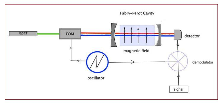
Figure 2: A highly over-simplified view of FPAS. Light from the laser passes through an electro-optical modulator (EOM) that and then enters the Fabre-Perot cavity where photons are converted to ALPs in the magnetic field (indicated by the black arrows). The intensity of the light that emerges from the cavity has an intensity modulated at the driving frequency of the EOM.
