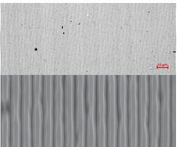
Images of MagAssemble transmission and reflection diffraction gratings. Top: Optical image of SiO2 lines with a square-wave profile and 1.5 µm trench depth. Bottom: SEM image of Si grooves with a triangular profile.
