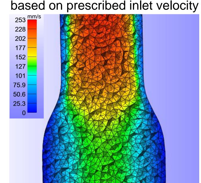
Fluid shear stress around the constriction
