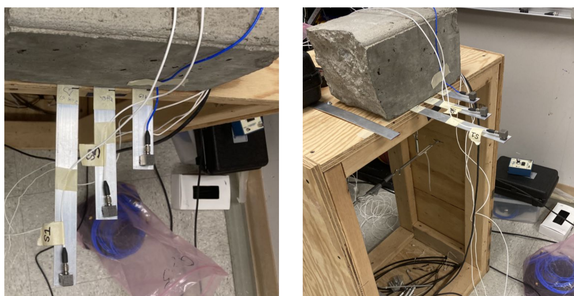
Constructed Resonator Mechanism
