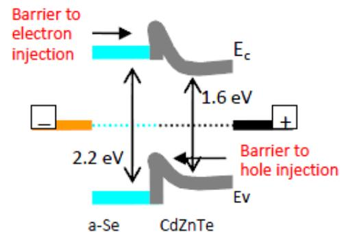
Figure 2. Band bending in metal/a-Se/ CZT Schottky contact concept
