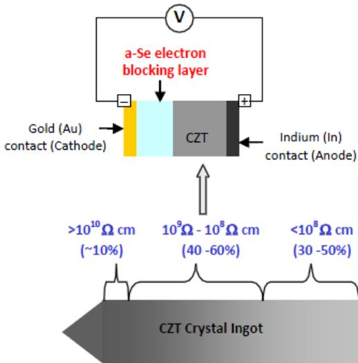
Figure 1. Proposed high barrier metal/a-Se/ CZT Schottky contact concept
