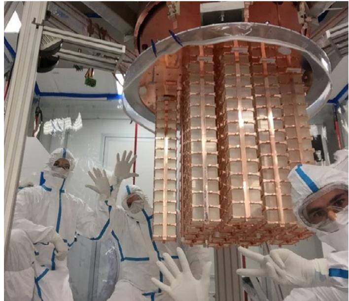
*The recently completed CUORE bolometer array shown earlier with two towers left to install.*
