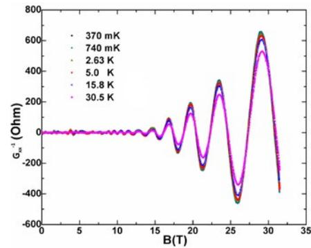
Figure 1: Temperature dependence of Shubnikov-de Haas oscillations in a sheet of graphene excised with an array of anti-dots. The isotherms are periodic in inverse magnetic fields and contain information about the Fermi-surface as well as quasi particle excitations.
