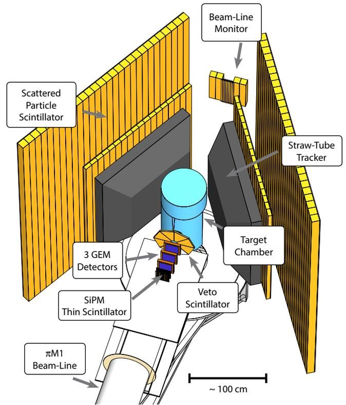
Figure 3: Rendering of the planned MUSE detector setup. The cartoon shows the setup as it is implemented in the MUSE simulation code, which our group has been developing. Our group is building the scintillation detectors (yellow) for the experiment at USC.
