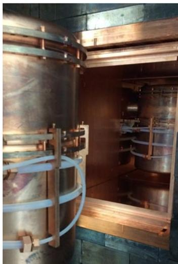
*MAJORANA Module #2 entering the shield where Module #1 is visible in the background.*
