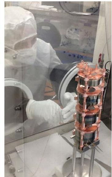
*The author testing a string of HPGe detectors. The electroformed copper making up the detector mountings was grown and machined underground at the Davis Campus of SURF.*
