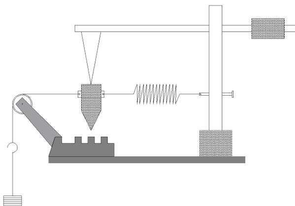
Figure 3: Measuring the force to stretch the spring.
