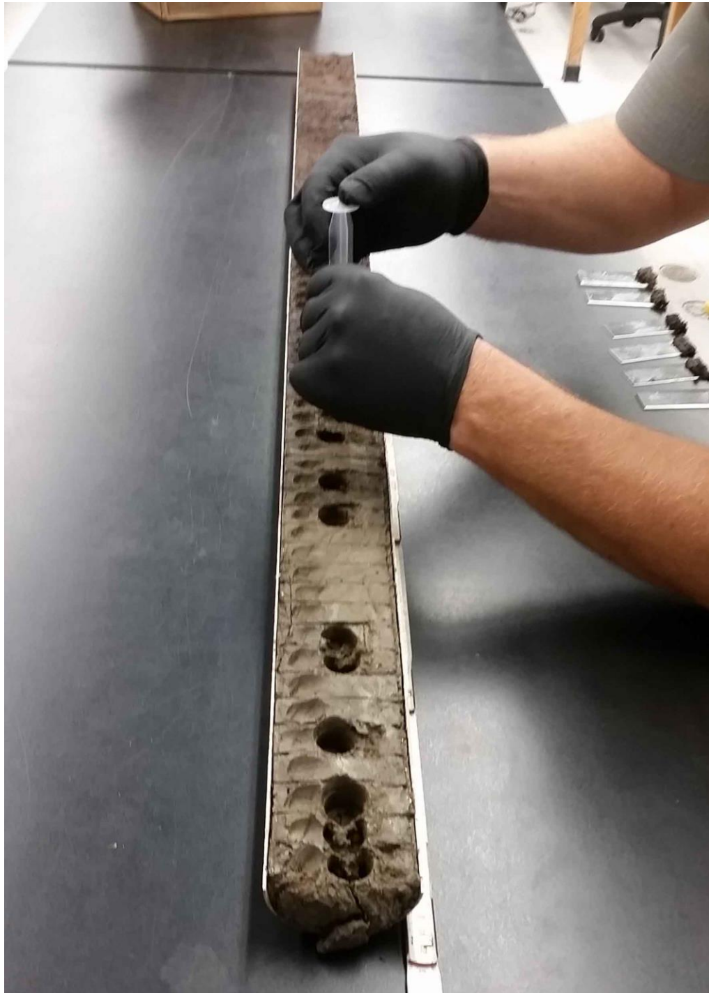
Figure II-9. Collecting core samples for environmental (eDNA) analysis.
