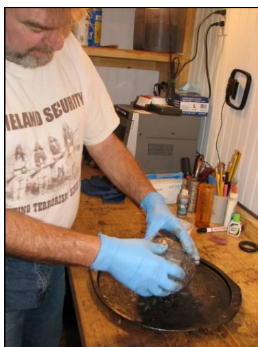
Image 3 Freddie Clark applying the Active Rust Primer
