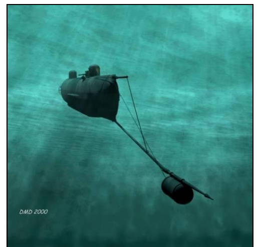
This image shows how the spar was connected to the submarine. A period diagram housed at the National Archives indicates that this Singer torpedo held 135 pounds of gunpowder.
