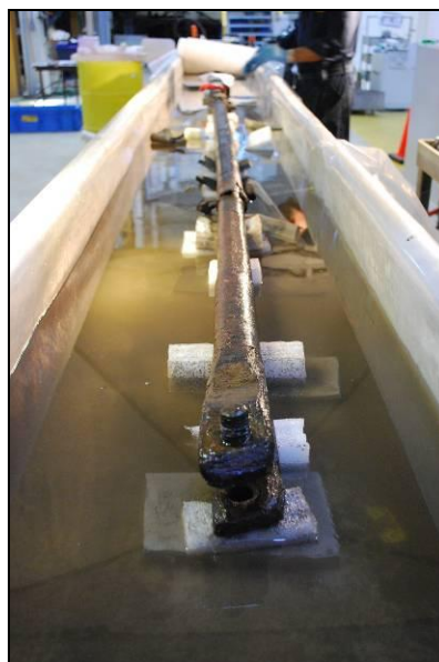
General view of the spar during deconcretion. The spar was a large pole that served as the delivery system for the Hunley 's powerful torpedo.
