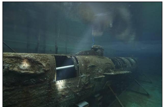
**Submarine after being rotated to an upright position. The Hunley tank will be filled with a chemical solution to begin the conservation treatment. (Copyright FOTH)**
