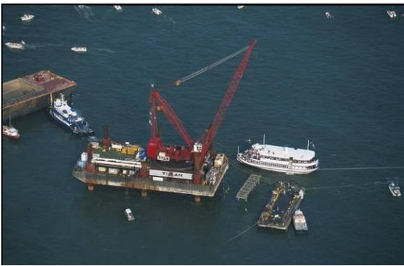
**The Hunley submarine in her truss being lifted by a crane to be placed on a barge. (Copyright FOTH)**
