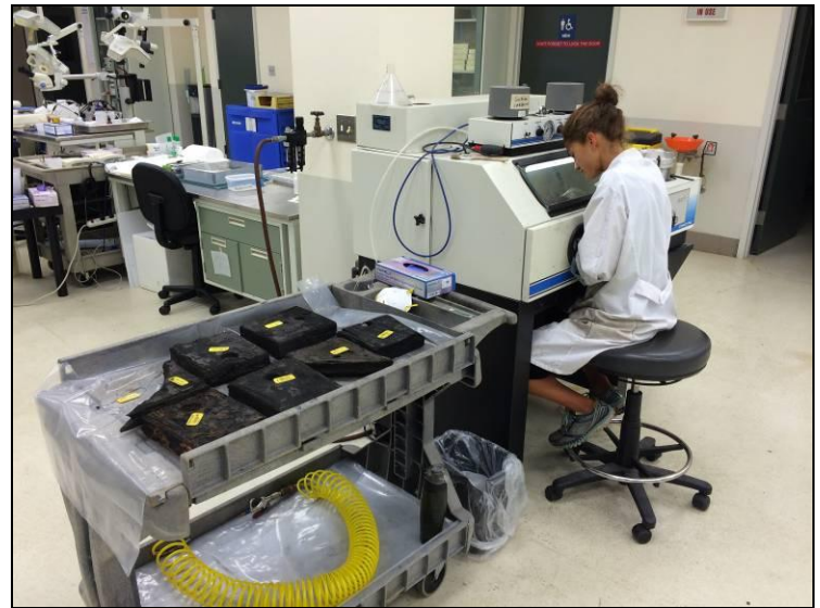
Figure 2. Conservator Virginia Ternisien using sodium bicarbonate abrasive to clean the surfaces of the ballast blocks. (Copyright FOTH)
