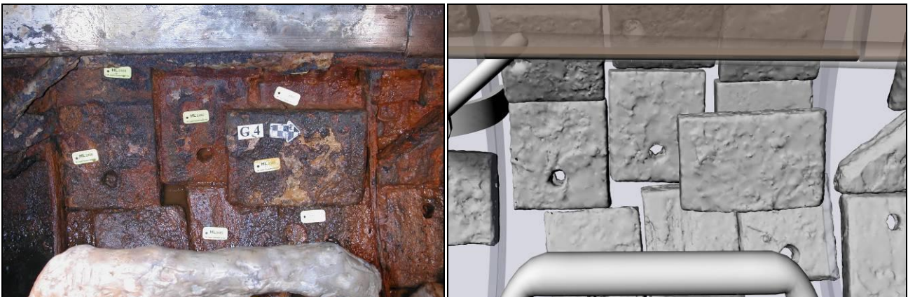
Figure 4. Close-up view of the corrosion pattern and cut marks (left) and a stamped mark on the side (right) of ballast block HL2449. (Copyright FOTH)
