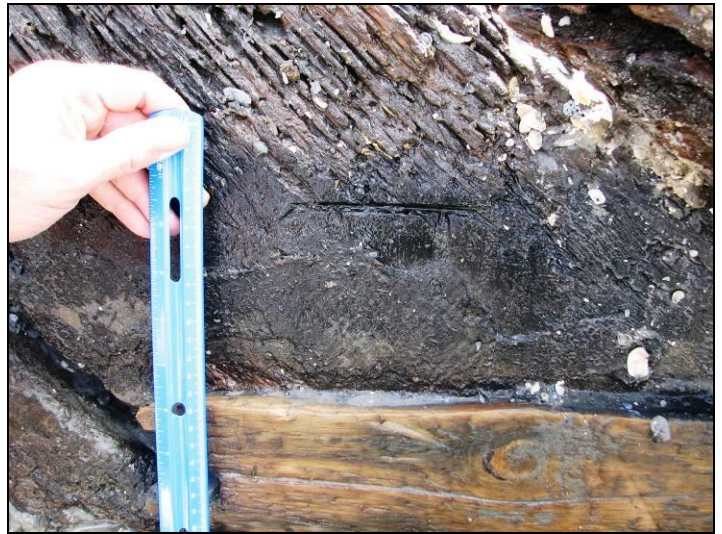
Close-up of the stempost area where sample fabric was taken. Note the draft mark and planking. (photo courtesy of SDAMP)
