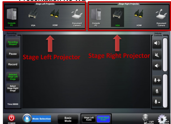
9. Select the source to be displayed on the left projector 10. Select the source to be displayed on the right projector By default console PC (podium computer) is selected
