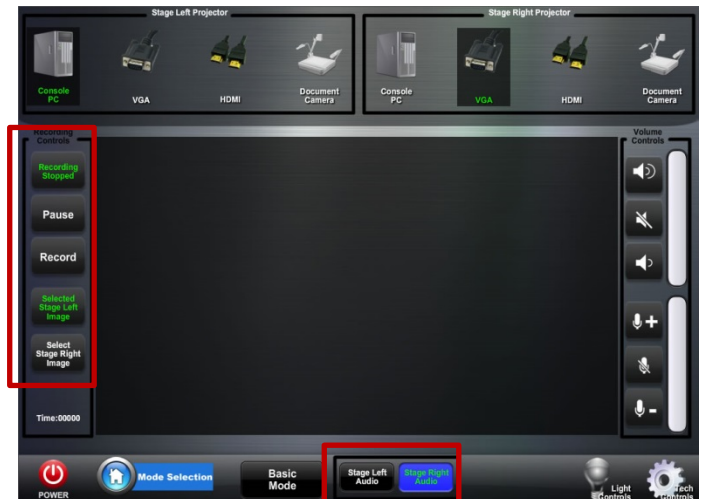
18. Select the audio to be recorded. By default the camera will record the audio source that has being selected for projection The camera in the room will not record the faculty member
