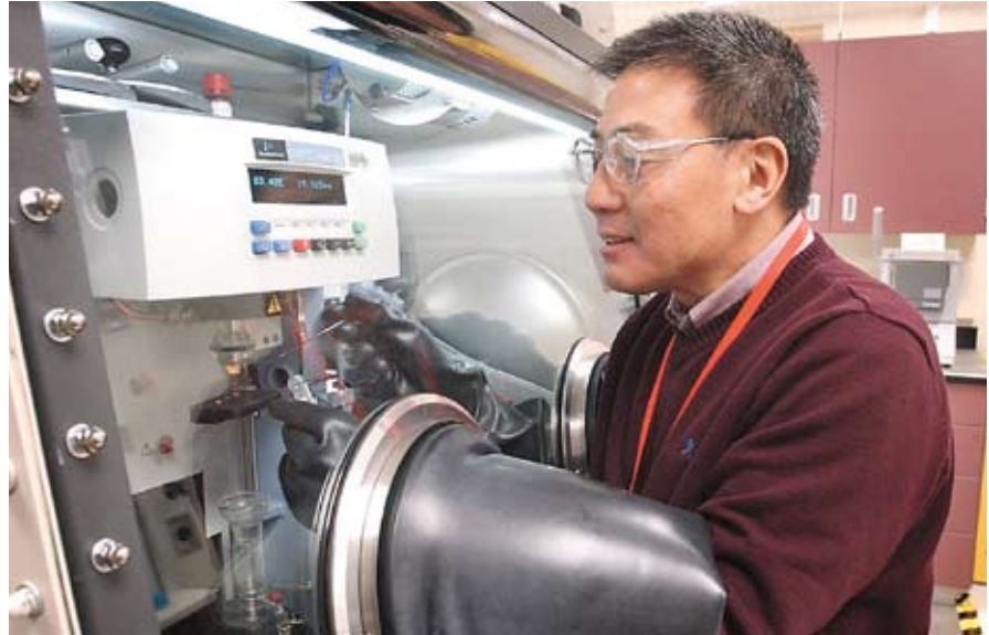
Ming Au, a principal scientist at the Savannah River National Laboratory in Aiken, measures hydrogen emissions at different temperatures. He does most of his work in the inert argon atmosphere of a glove box. Photo by Tim Dominick The State
